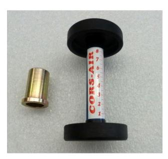
Using a well balanced propeller is very important for the duration of your engine. We offer a very simple tool to check and correct the balancing of your propeller.
