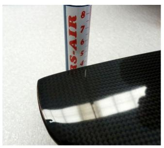
Check at which height the first tip of the propeller arrives, then rotate the propeller on the central pin without moving the ruler and check the height of the second tip
