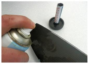
If you find a different height for the two tips, it means that the propeller is unbalanced, so spray on the lighter tip (the one that stays higher) some transparent paint, until they reach the same height
